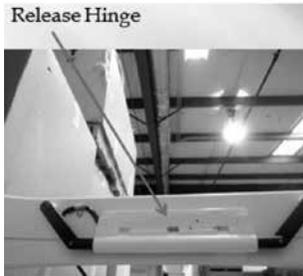
1. If the hatch was opened with the lid in the fully closed position, the release hinge will still be in the down position.
