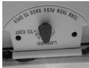
8. The red knob should be in this position during normal operation of the vehicle.
