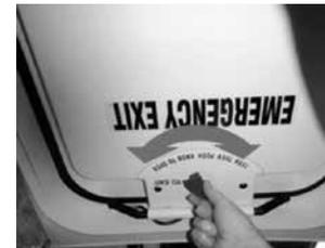
1. Rotate the red knob 90 degrees in either direction.
