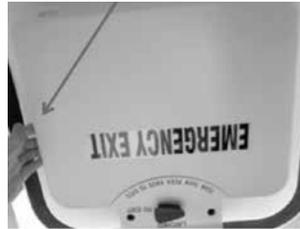
6. Grasp both sides of the lid and pull down to fully close the hatch.
