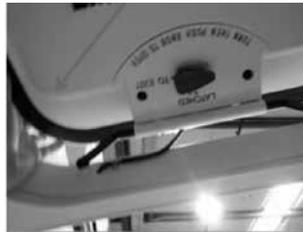
5. Pull down on the top of the lid to force the release hinge and the lid together until you hear “clicks.” This will be the spring loaded handle setting in place.
