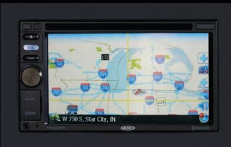
A Jensen touch-screen AM/FM radio with CD/DVD, bluetooth, back-up camera, and GPS provides easy navigation for the driver.
