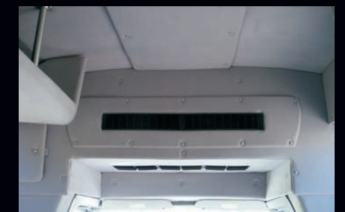
Passenger area air conditioning is located above the driver's area of the bus to maximize head room at the rear of bus
